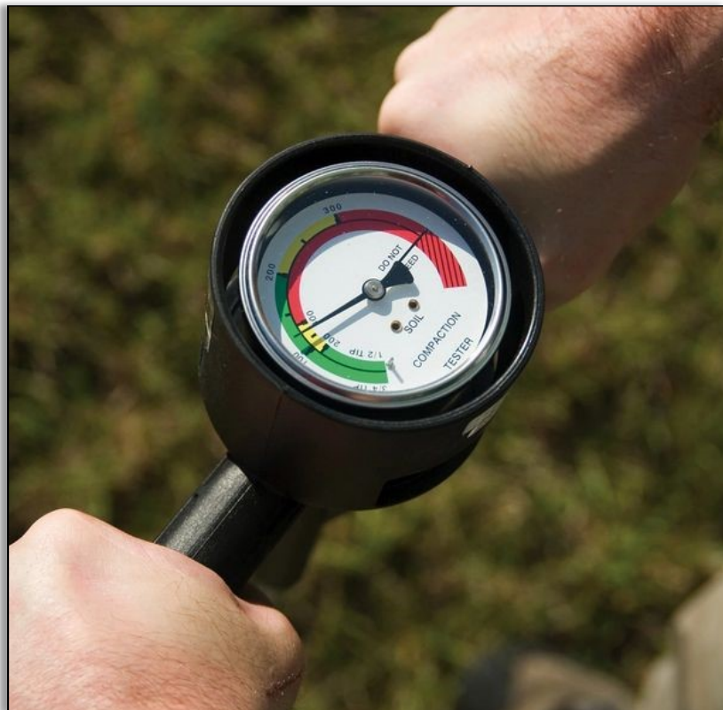
A soil penetrometer can measure the soil compaction.
